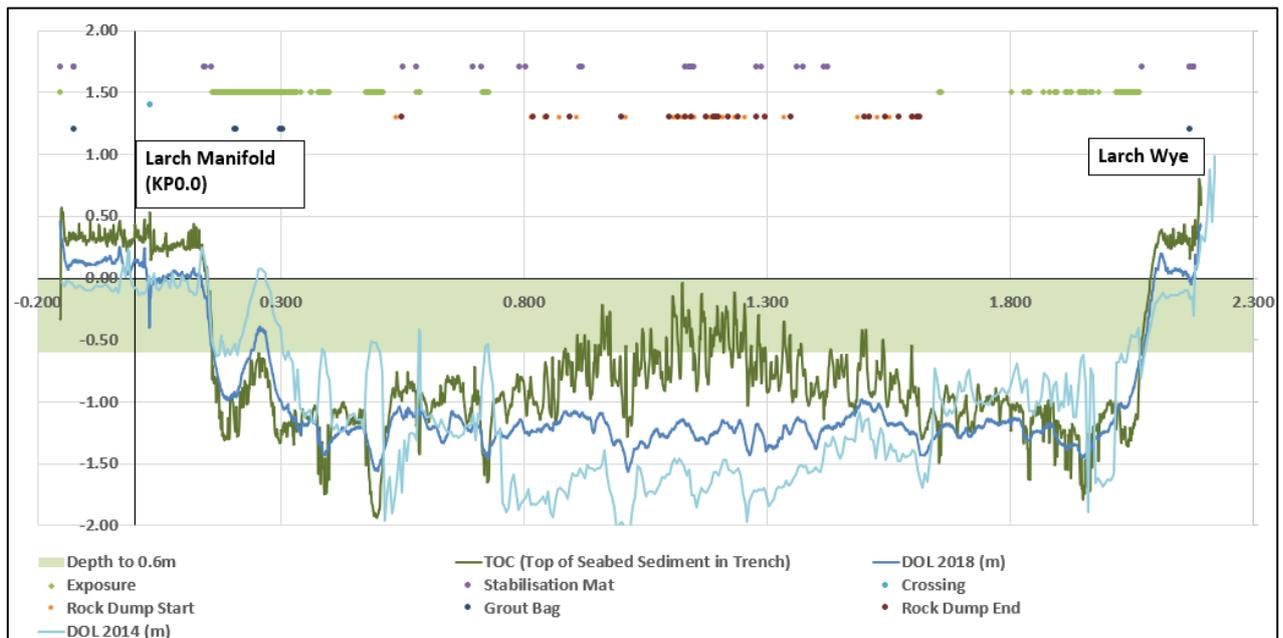
Figure 3-5: PL1527 10" Production Pipeline Burial Profile (2014 & 2018)
