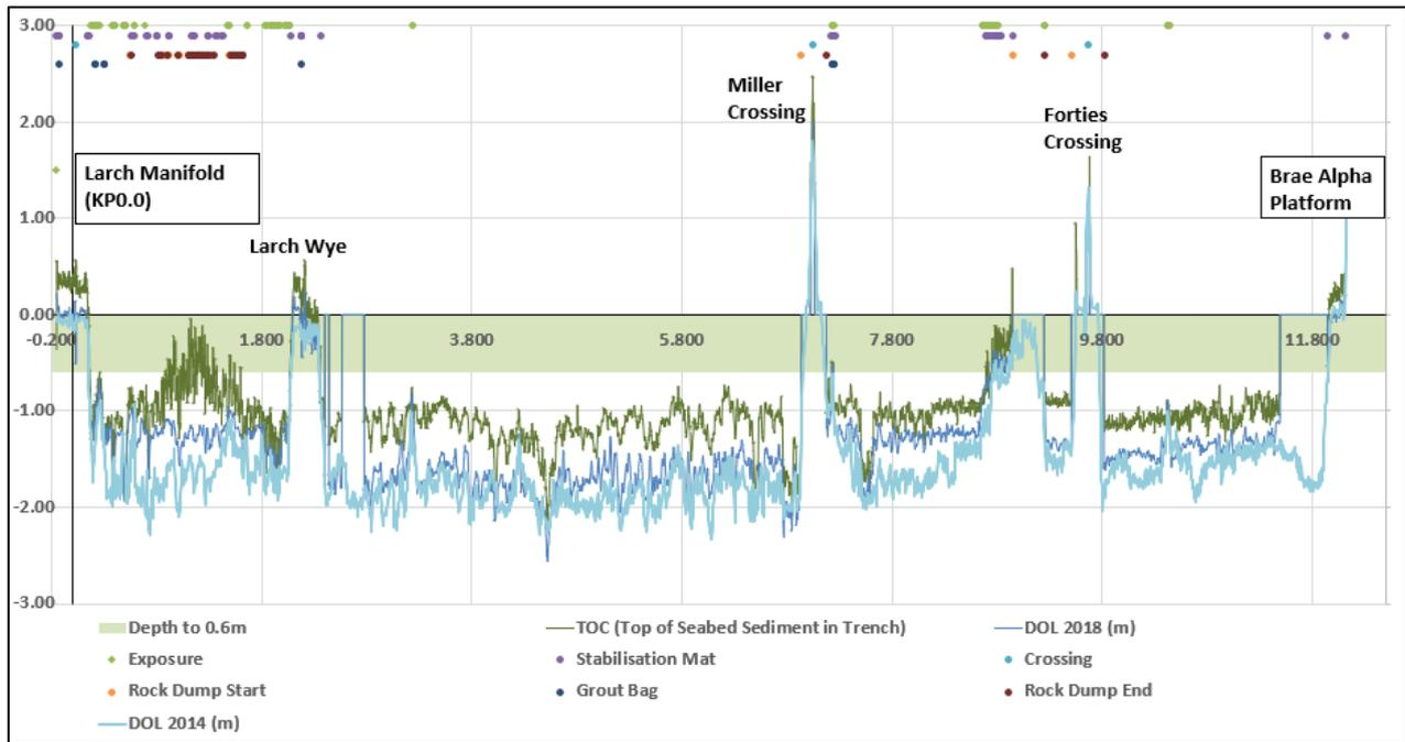
**Figure 3-6: PL1531 4" GL Pipeline Burial Profile (2014 & 2018)**
