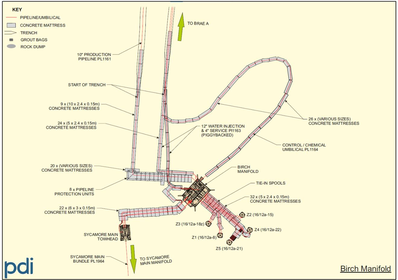
Figure A-5: Birch Manifold and Wells
