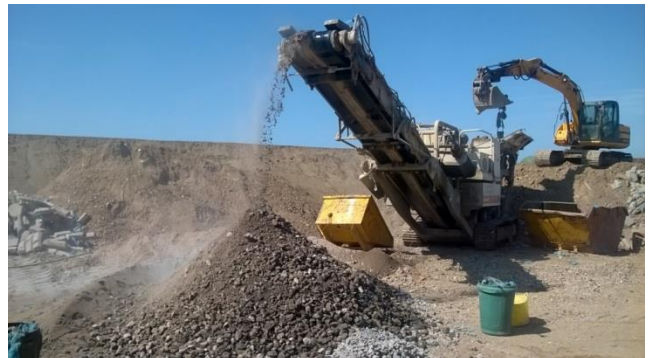
Figure 9.6.1: Concrete mattresses finally crushed and recycled
