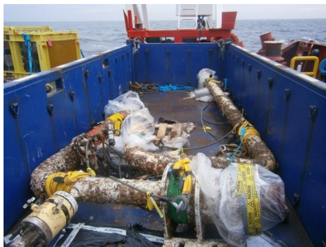
Figure 9.4.1: Pipe spools stored inside container
