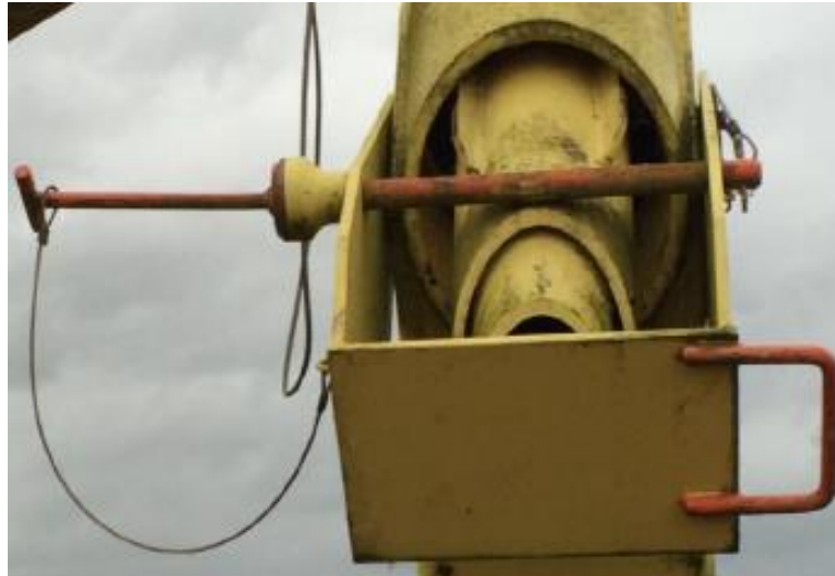
Figure 4.2.2: Trawl Legs Locked in Retention Bucket
