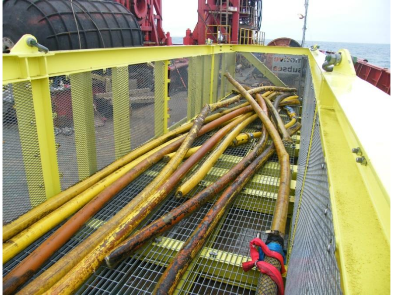
Figure 9.5.2: Umbilical sections stored in basket
