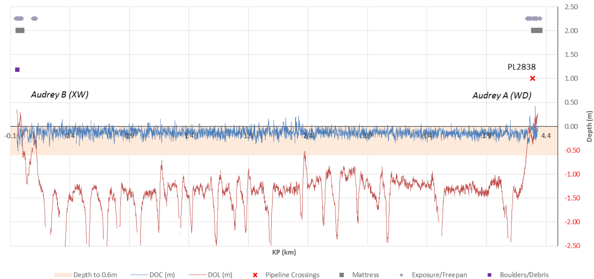
PL723/4 14" Gas Export / 3" Methanol Line Burial Profile (DOB & Events from 2016)
