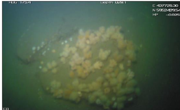
Figure 4-10: Example of grout with encrusting fauna attached
